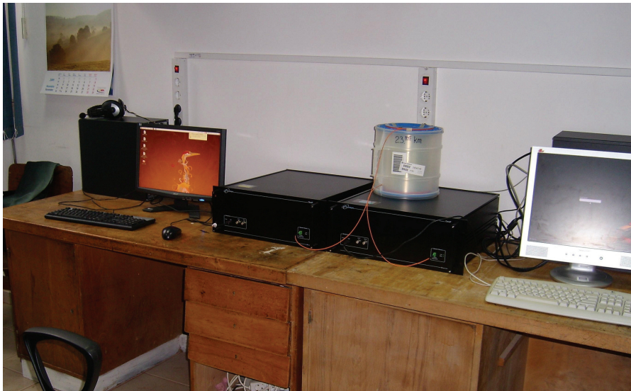
Fig. 12. Communication line setup used in the QUANTGRID D11-044 project (Inst. for Laser and Plasma Phys. – Bucharest), with its two dedicated computers (Bob – receiver and Alice – sender). The quantum channel (23.845 km) optical fiber spool is on top of the Bob station. The classical channel linking the computers is local LAN Ethernet.
